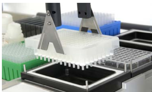
Fig. 1: Xiril X100 Automated Liquid Handling System equipped with gripper tool and Solid Phase extraction unit.
